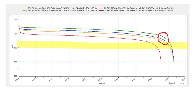
**LiFe battery can be permanently damage if discharged below a critical voltage**. If using the FlySky-i6 Transmitter/Receiver combination, the user is advised to set the receiver battery alarm voltage to 5.5v and to prevent battery under-volt damage the battery disconnect voltage should be set to 5.0v.
